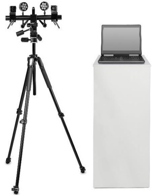
Figure 1(a) The illuminating light focusing on the sample before calibration 1(b) The figure represents the 3D camera mounted on tripod and the system to compute data for the test of specimen.
